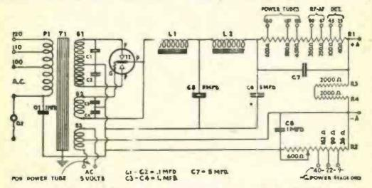
for efficient tube operation. A vacuum tube, to operate at maximum efficiency. either as RF amplifier, detector or AF amplifier, must have a certain definite relationship between the plate voltage and the blasing grid voltage. In other words, if your RF tube is to perform efficiently as an RF amplifier without distortion you must maintain the B-O relationship.
